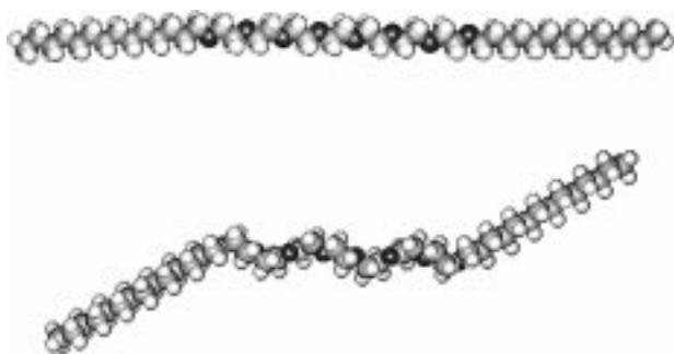
Figure 3. Oligomer structure obtained by crystallization from methanol (top) and hexanes (bottom).
